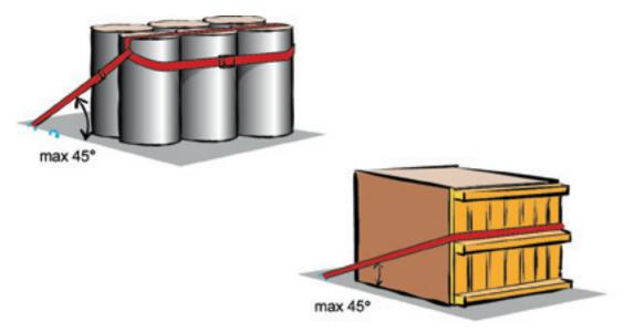
The spring lashing can be done in many ways. However, if the lashing is not applied to the upper edge of the cargo item, the tipping limits of the cargo weight is reduced.
