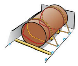
A loop lashing will secure a cargo item on each side with a pair of webbings. At the same time the cargo will be prevented from tipping. At least two loop lashings per long cargo item should be used.
