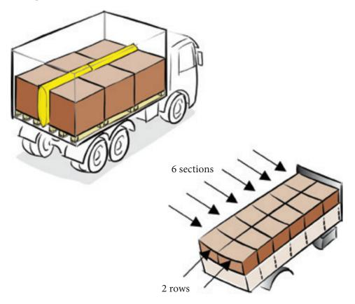
If the cargo is only bottom blocked, lashing may be needed to prevent tipping, see the tipping tables in this Quick Lashing Guide.
