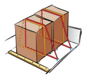
If the cargo item contains more than one section and the sections support each other and stop any twisting from occurring, then only one loop lashing per section of the cargo, may be needed.
