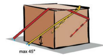
This spring lashing set-up has two legs on each side, which secures twice the weight that is indicated in the table.
