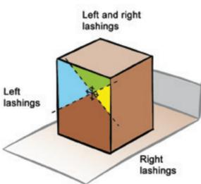
The areas where you can attach lashing straps are limited by two straight lines running diagonally through the centre of gravity at an angle of 45°.
