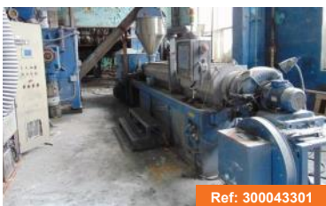
Twin-screw extruder for PVC compounds (2012) BAUSANO MD 125/30R Screw Diameter: 125 mm Throughput: 800 kg/h Screw L/D Ratio: 30
