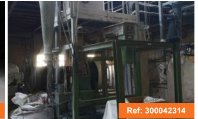
Pulverizer (1995) PREVIERO PD 300 Output Capacity: 450 kg/h Disc Diameter: 300 mm
