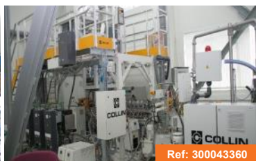
Twin-screw extruder for other materials (2008) COLLIN ZK 35 Screw Diameter: 35 mm Screw L/D Ratio: 56
