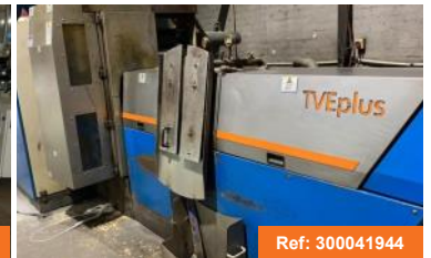
Single screw repelletizing line (2009) EREMA 1310 TVE Plus Screw Diameter: 100 mm Output Capacity: 500 kg/h
