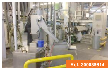
Twin-screw extruder for PE/PP compounds (2001) LEISTRITZ ZSE 50GL - 36D Screw Diameter: 50 mm Throughput: 120 kg/h Screw L/D Ratio: 36
