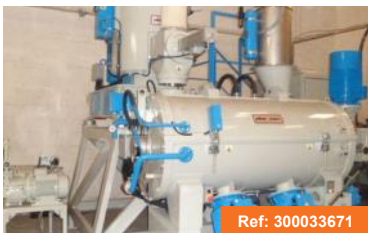
Combination mixers (2012) PLASMEC COMBIWOOD-HC/300/1000/FV/W-PP/PE Mixing Capacity: 300 l Cooling Capacity: 1000 l
