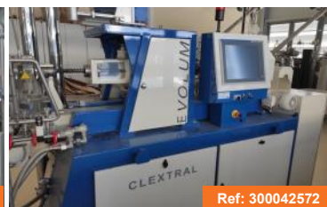
Twin-screw extruder for other materials (2015) CLEXTRAL EV 25 Screw Diameter: 25 mm Screw L/D Ratio: 24
