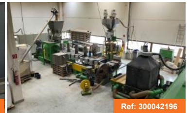
Compounding extrusion lines (2005) LEISTRITZ, REIFENHAUSER HFL 110/48 - HFL 50/20 Complete production line for PROFILES: WPC, plastic RPC or plastic SPC
