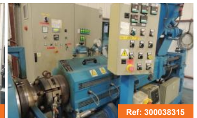
Twin-screw extruder for PVC compounds (2003) AMUT BA 72 Screw Diameter: 72 mm Throughput: 180 kg/h Screw L/D Ratio: 22
