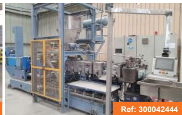
Twin-screw extruder for PE/PP compounds (1993) WERNER & PFLEIDERER ZSK 70-36D Screw Diameter: 70 mm Throughput: 500 kg/h
