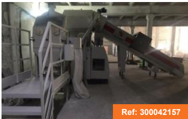
Single screw repelletizing line (2018) STARLINGER RecoSTAR universal 65 VAC Screw Diameter: 65 mm Output Capacity: 150 kg/h Screw L/D Ratio: 40
