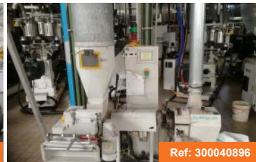
Single screw repelletizing line (2013) PLASMALPHA Alpha 45 Screw Diameter: 45 mm Output Capacity: 40 kg/h
